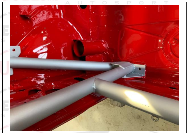
PHOTO 6 FRONT ROLLBAR TO FLOOR ATTACHMENT
