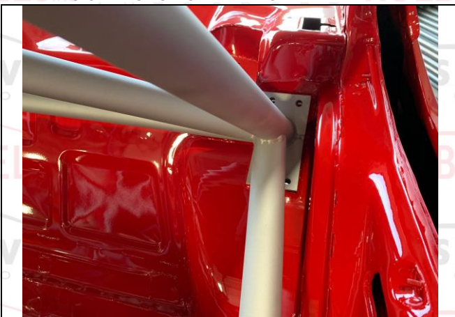
PHOTO 5 REAR BACKSTAY TO BODYSHELL ATTACHMENT
